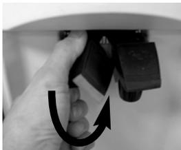
13. Re-install the floater. Make sure that the opening of the floater faces upwards.
