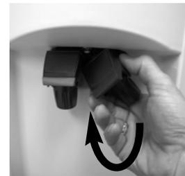
\* The warm-water faucet (white tab) or the hot-water faucet (red tab) goes in the left hand socket (facing the cooler). Insert with nozzle at 270°, push hard and turn counter-clockwise.
